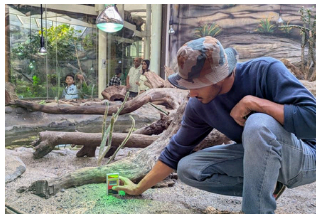
UV index meter used to measure the ultraviolet radiation at a basking spot at the reptile enclosure.
