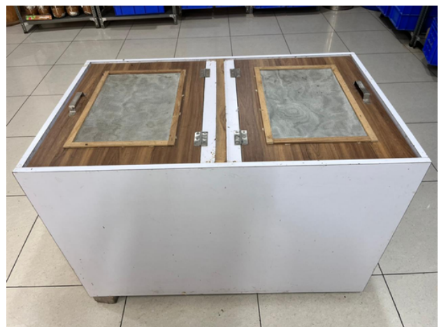
Wooden roach culture box with mesh-covered lids, designed to provide ventilation while allowing secure containment and routine monitoring.
